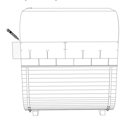
**STEP 33:** Remove protective film from the bottom of the sheet. Third row goes exactly like first row. Cut half rectangle from shingle and fix it with shingle nails.
