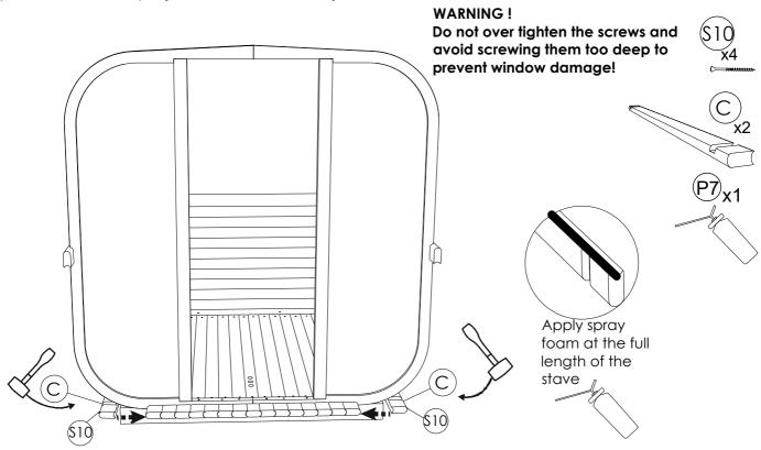
**STEP 10**: Fix 12 stave (SC) on both sides with screws (S10). Use rubber hammer for tighter placement. Use foam between every stave. When both corners are done, take of connecting staves.
