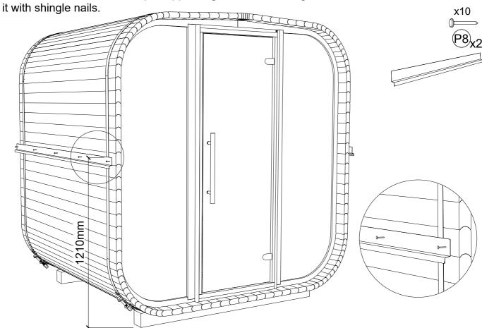
**STEP 28:** Fix underlay on the both sides first. Upper underlays overlaps no less then 100mm on both sides. Leave underlay about 40mm over the back and front edge, make sure it's evenly on sides too.
