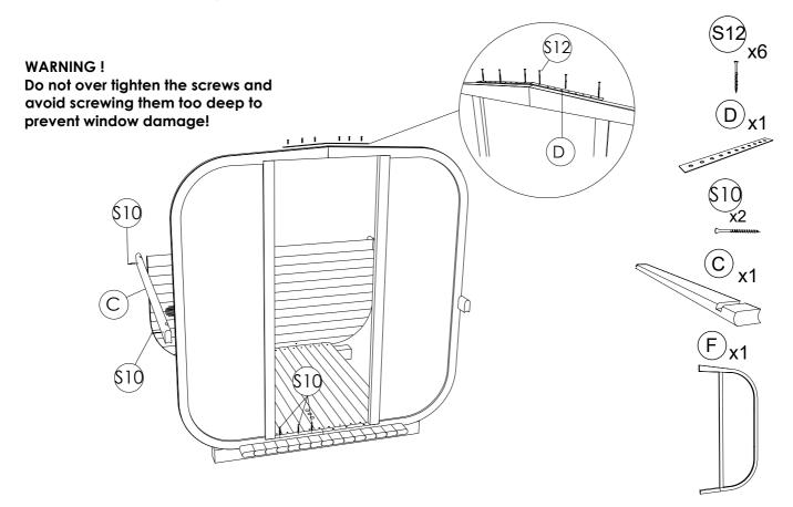
**STEP 9**: Fix one stave (C) on both sides with screws (S10). Use rubber hammer for tighter placement. Use spray foam between every stave.
