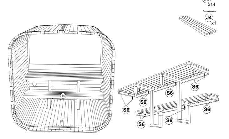
**STEP 25**: Install bench legs (J1;) with (S6) screws. The left leg needs to be installed next the front panel (F), right leg is 750mm from bottom rear panel. Fix sauna bench (J8) using (S6) screws.
