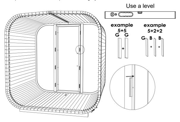
**STEP 20:** Fix one side of the door box with screws (S14) slightly to the outside through spacers. Then put spacers in other side. Combine spacers for necessary width. Spacers must fit tightly, they can't slip down before door is fixed with screws. Use screws (S14) to fix doors. Check door box, both sides should be straight, they must not be bent inwards or outwards.
