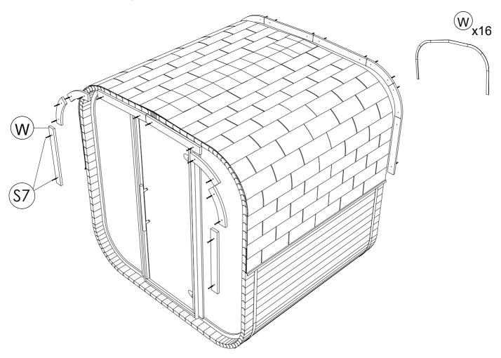
**STEP 38:** Use bitumen sealant behind decorative boards to fill gap between shingles and boards.
