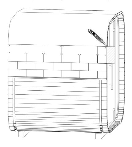
STEP 34: Keep placing shingles till last layer goes over the middle of the roof.
