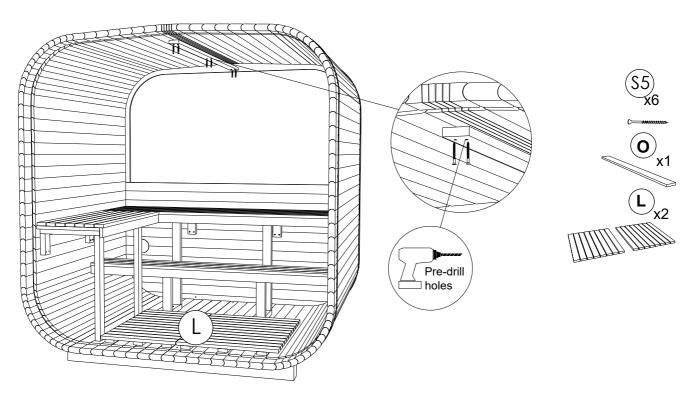
**STEP 27**: Place the rain droplet upper edge 1210mm from ground. Make sure it's leveled. Fix it with abjude noils
