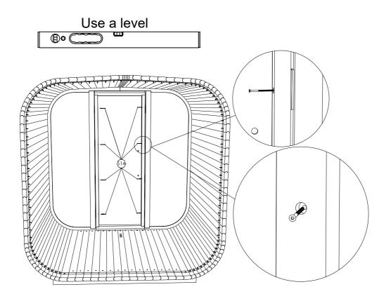
**STEP 21:** Use spray foam around door box. Let the spray foam dry. The excess amount will come off easily if you don't touch it while it's wet. Fix door moldings to both sides and on top of the door with (S5).
