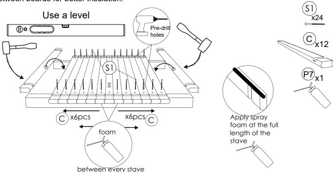
**STEP3:** Drill fourteen 10mm holes in front and back wall groove to the out-side in board connections as shown in the picture. This will help drain excess water faster.
