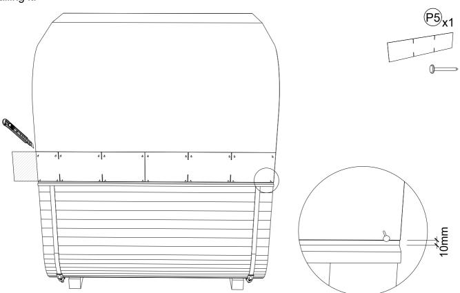
**STEP 31:** Remove protective film from the bottom of the sheet. Start placing shingles over starting shingles. Cut half of the rectangle from whole shingle and fix it with nails. Fix next shingle next to first.
