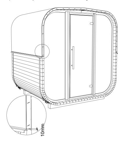
**STEP 30:** Remove protective film from the bottom of the sheet. Place starting shingles next to each other. Then fix with nails as in picture. Cut excess part of the starting shingle before nailing it.
