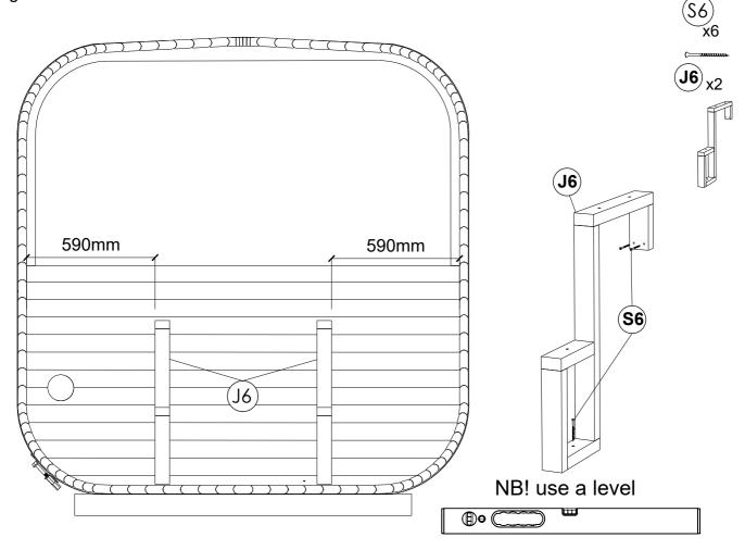
STEP 23: Place long sauna bench upwards on the bench legs. Then install bench support boards (J3) on the side walls using S6 screws, at the same level as the bench legs. leave gap from back wall about 20mm.
