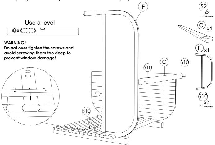
**STEP 8**: Place the second front panel (F). Slide it together that the top and bottom connects. Fix it at the panel threshold with screws (S2). Make sure it's level. Use metal bracket on top of the front panels to fix them together.
