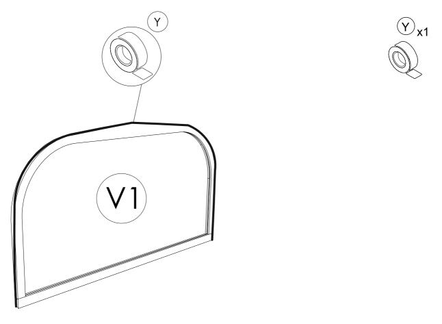
**STEP 13**: Install the panoramic panel (V1) with caution. Use foam between panels for better insulation. Place it on top of the lower back panel (V). Check level and that side edges are aligned with bottom panel. One keeps holding the panel, and the other is fixing the side stave on a curve using screws (S10). Secure the panel (V1)with screws at the both corners using two screws (S4).
