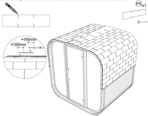
**STEP 37:** Install front and back decorative roof finishing boards using (S7). Start by fixing two top boards, then rest of it goes next to each other.
