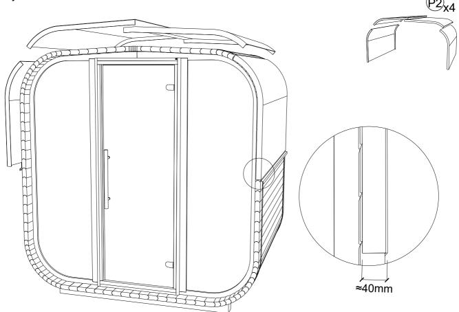
STEP 29: Staple underlay at the front and back edges. Cut excess underlay if necessary.
