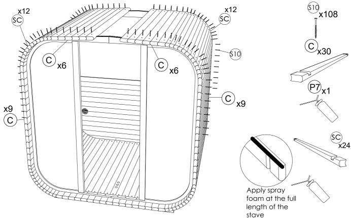
**STEP 15**:Finish roof with the 2 (C) staves and final staves (H). If needed, use thinner staves (H1) to fil the gap between (H) staves and apply foam between staves. Make sure that centre of the roof is tightly filled, then fix with screws (S10).
