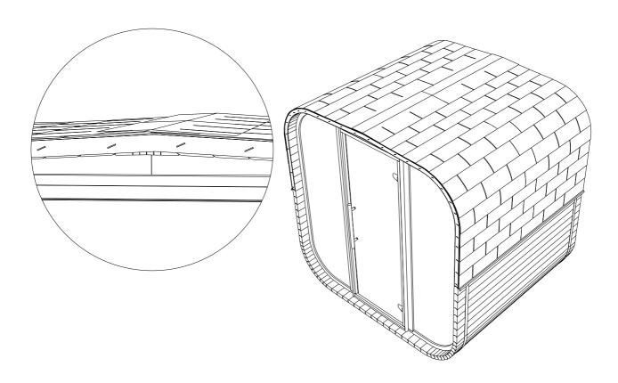
**STEP 36:** For top of the roof use starting shingles. Cut some shingles in squares, there are marked lines. Take off protective film. Nail each shingle with two nails. Next shingle goes about 160mm over previous. After it's done, use heat source for better adhesion.
