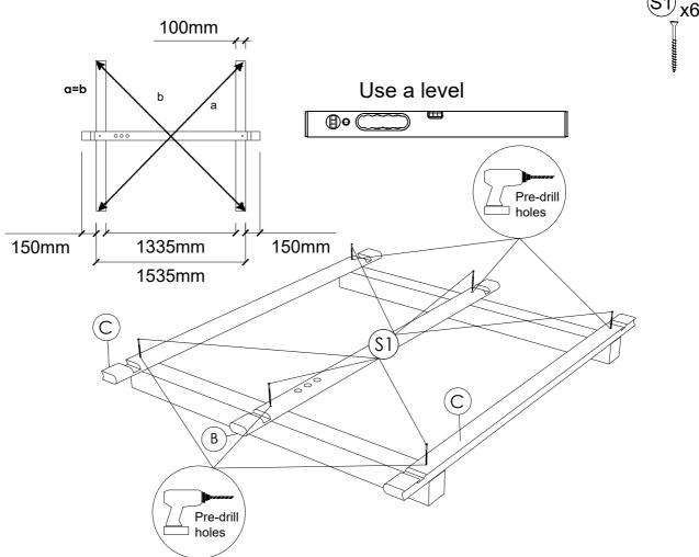
**STEP 2:** Fix 10 staves (C) to each side from the center stave. Check level while installing staves and use rubber hammer for tighter placement. Pre-drill holes for screws. Use spray foam between boards for better insulation.
