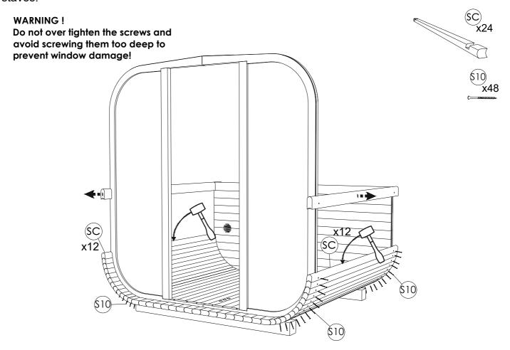
**STEP 11**: Fix one stave (C) on both sides with screws 4x60 (S10). Use rubber hammer for tighter placement. Use foam between every stave. When both corners are done, take of connecting staves. Keep fixing staves till reach top of the rear panel (V).
